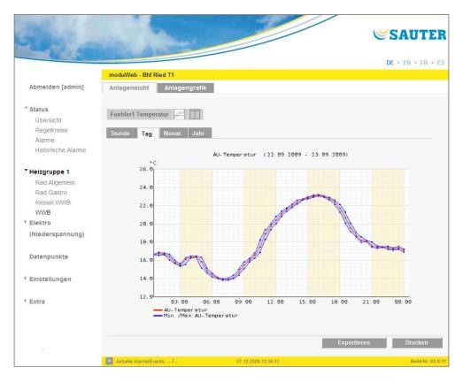
SAUTER EY modulo 5 ideally meets the requirements for this project without a management level thanks to its **modular design**, its extensive **local operating options**, and remote operation and alarms with **moduWEB**.
