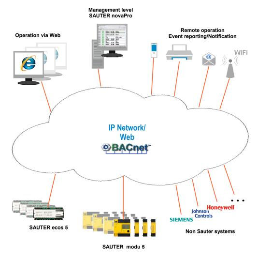
The modu 5 automation and room management stations are the core of this complete system range for regulating, controlling and monitoring building services installations.
