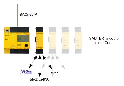
up to **2 moduCom** modules can be plugged in to each modu525 AS. They must be inserted in positions 1 and 2. The modu525 can also be expanded in the normal manner by adding more I/O modules so that plant devices can be connected directly (max. 6 or 7 units, max. 148 I/O, up to 512 BACNet objects in total).
