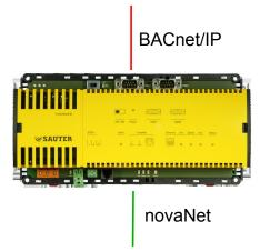
The **moduNet300 application master (AM)** integrates the SAUTER EYmodulo 2 automation stations and room controllers (as well as EY3600 stations) connected via the novaNet into the open, standardised BACnet/IP communication protocol.
