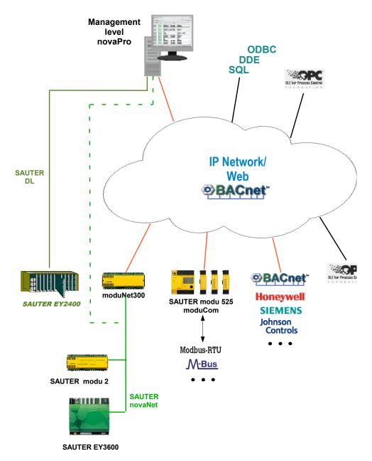
Because it is a **BACnet** system, **SAUTER EY-modulo 5** is theoretically open for direct integration with all third-party BACnet equipment systems or with third-party systems which can connect to BACnet (such as gateways).
