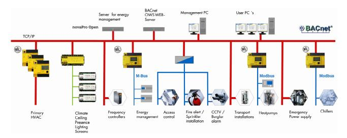
SAUTER EY modulo 5 ideally meets the high requirements for this project thanks to its **high performance**, **modular design** and wide range of open **communication options** via BACnet/IP and moduCom.
