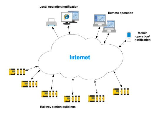
• Cost-optimised connection to the internet via a router with a USB-UMTS stick in each railway station.
