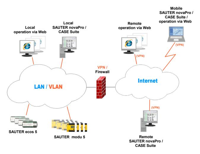
In principle, **BACnet/IP** can be operated **in any IP network**. (In addition, the **moduWeb** functions of the AS (operation with browser and e-mail) generally integrate into every IP-LAN / WAN / internet environment with no problems.)
